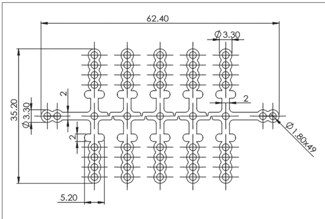
▲ **Appendix Fig 1** Structure of the titanium frame.
